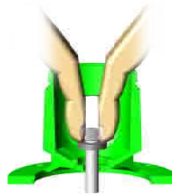
Figure 18 - Press In Seal
